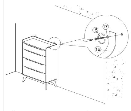
5. Finally, attach safety strap (16) and washer (17) using 4x30mm screw (15) to the wall.
