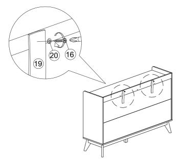
4. Add safety strap (19), washer (20) using 3.5x15mm screw (16) to back of cabinet.
