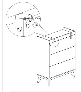
4. Add safety strap (16), washer (17) using 3.5x15mm screw (13) to back of cabinet.
