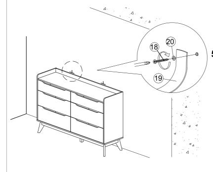
5. Finally, attach safety strap (19) and washer (20) using 4x30mm screw (18) to the wall.
