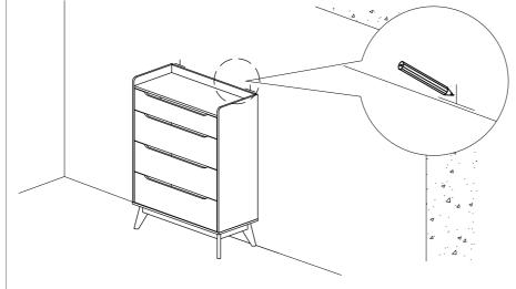
1.First mark the wall with pencil as in diagram.
